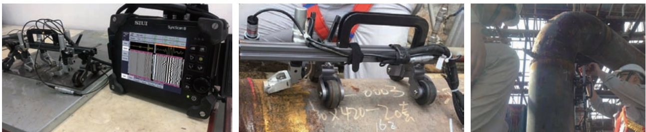
Phased array & TOFD crawler
